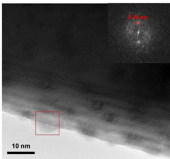
**Fig. 5.** HRTEM image of a nanowire fragment decorated with randomly distributed 5–10 nm tin oxide nanoclusters, FFT pattern from the red square in upper right inset indicates 0.34 nm lattice fringes, which are consistent with a (1 1 0) reflecting plane of the tetragonal polymorph of SnO<sub>2</sub>. (For interpretation of the references to color in this figure legend, the reader is referred to the web version of the article.)
