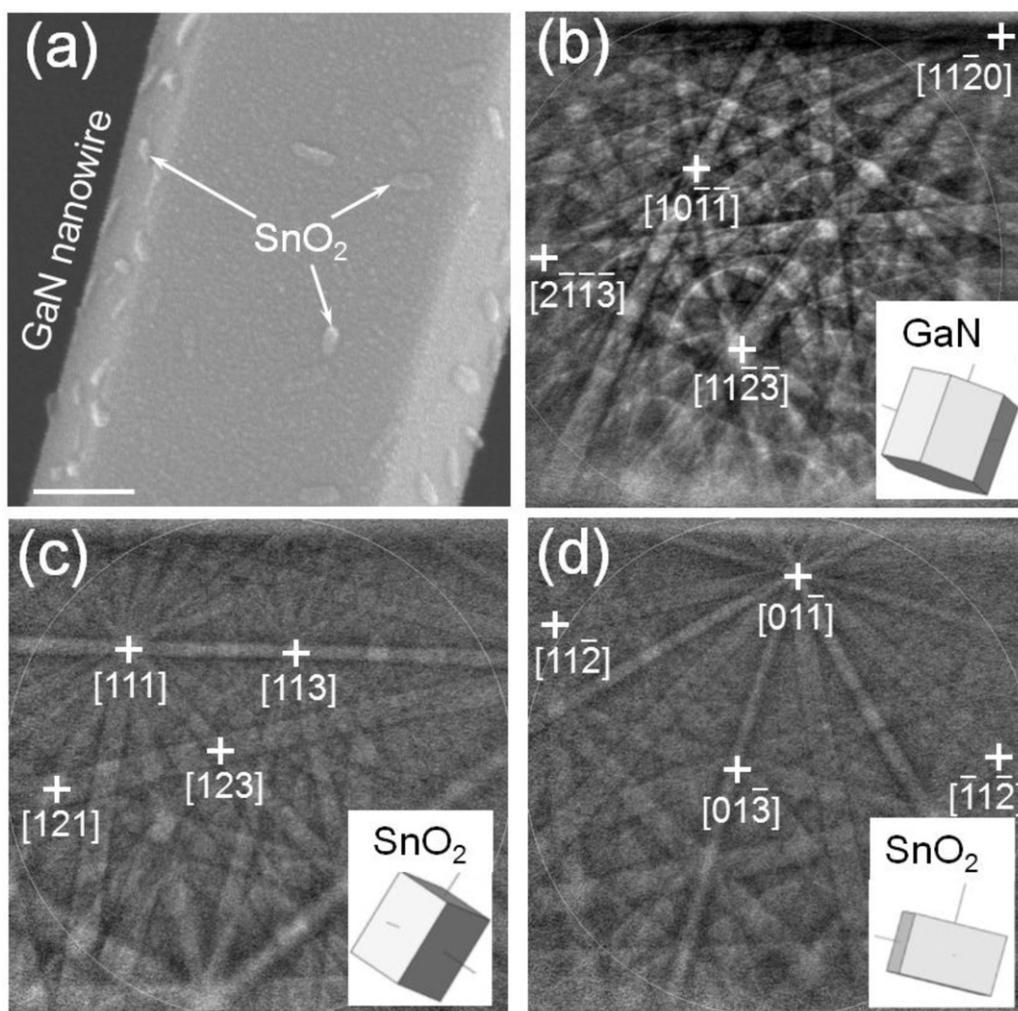
**Fig. 4.** FESEM image of the nanowire fragment decorated with tin oxide nanoparticles (a); EBSD patterns of GaN (b) and SnO<sub>2</sub> (c–d) with simulated unit cells in the insets. Unit cells in (c) and (d) indicate random crystallographic orientation of SnO<sub>2</sub> grains on GaN surface. Scale bar in (a) is 100 nm.
