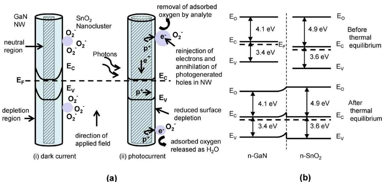
Fig. 8. (a) Schematic representation of sensing mechanism of SnO<sub>2</sub> coated GaN nanowire hybrid sensor. (b) Band diagram of SnO<sub>2</sub>/GaN heterojunction.
