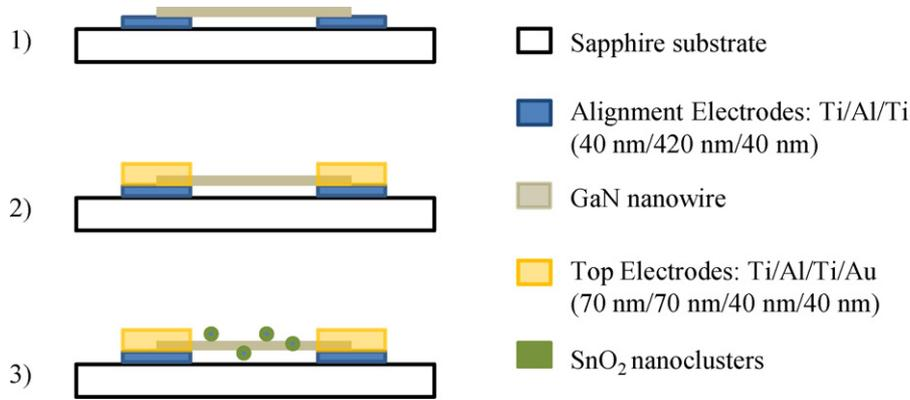
Fig. 1. Fabrication steps for the SnO<sub>2</sub> nanocluster coated GaN nanowire alcohol sensor.
