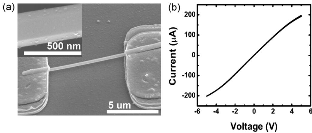
Fig. 2. (a) FESEM image of a GaN suspended bridge structure. Inset shows nanowire facets with tin oxide nanoclusters (b) dark  $I$ - $V$  characteristic of the GaN nanowire sensor coated with SnO<sub>2</sub> nanocrystals after RTA at 700 °C for 30 s in argon.
