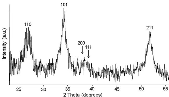
Fig. 3. XRD  $\Omega$ - $2\Theta$  scan of a 40 nm thick SnO<sub>2</sub> film after 700 °C anneal in argon for 30 s. Indices correspond to tetragonal SnO<sub>2</sub> phase (P42/mmm) with  $a = 4.758(3)$  Å and  $c = 3.175(2)$  Å lattice parameters.
