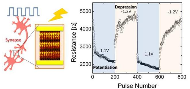
Fig. 11. Synaptic device from an MoTe<sub>2</sub> RRAM.
