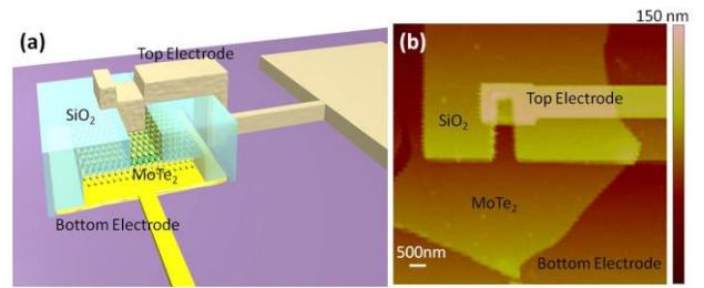
Fig. 2. (a) Schematic diagram of a vertical metal/MoTe<sub>2</sub>/metal device. (b) AFM image of a vertical MoTe<sub>2</sub> device.
