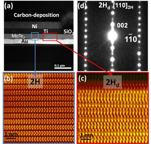
Fig. 5. (a) HAADF-STEM image showing the cross-section of a MoTe<sub>2</sub> device. Higher magnification HAADF image from the region defined by the blue/red box in (a) showing (b) 2H and (c) a distorted structure (2H<sub>d</sub>) taken along the [110]<sub>2H</sub> zone-axis. (d) Corresponding nano-beam diffraction pattern taken from the distorted 2H<sub>d</sub> area.
