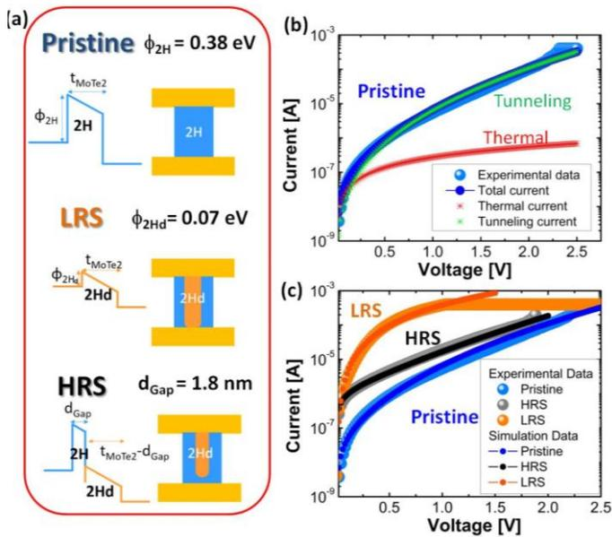
Fig. 8. (a) Schematic band diagrams of the RRAM in its various states. (b) Experimental and simulation data of a pristine device. (c) Experimental and simulation data for the LRS, HRS and pristine state.
