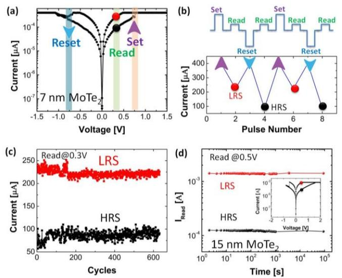
Fig. 9. (a) DC characteristic of a 7 nm thick MoTe<sub>2</sub> layer RRAM device. (b) shows the various current levels after pulse switching. (c) Current versus cycle in the LRS and HRS at a read voltage of 0.3 V. Current compliance is set to 400  $\mu$ A. (d) Retention of the HRS and LRS for a 15 nm thick MoTe<sub>2</sub> RRAM device. Current compliance is set to 1.2 mA.
