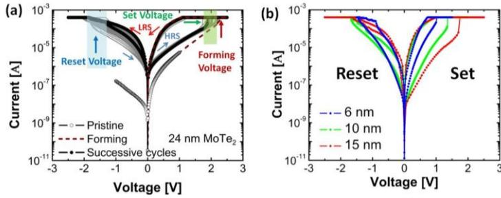
Fig. 3. (a) I-V curves of a 24 nm MoTe<sub>2</sub> device with an active area of 330 nm x 500 nm. 40 cycles are shown in the grey line curves. Current compliance is set to 400  $\mu$ A. (b) I-V curves of vertical MoTe<sub>2</sub> RRAM devices from 6 nm, 10 nm, and 15 nm MoTe<sub>2</sub> layers with active areas of 502 nm x 360 nm, 522 nm x 330 nm and 500 nm x 330 nm respectively. (c) Forming/Set voltage values scale with the MoTe<sub>2</sub> thickness.
