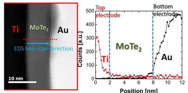
Fig. 6. EDS line-scan analysis of the filament region of a device in its LRS. Little Ti/Au signals were detected in the filament region due to ion-milling contamination during sample preparation.
