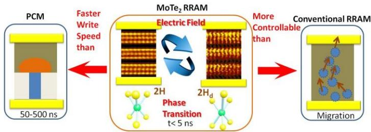
Fig. 1. Highlight features of the MoTe<sub>2</sub> based RRAM.
