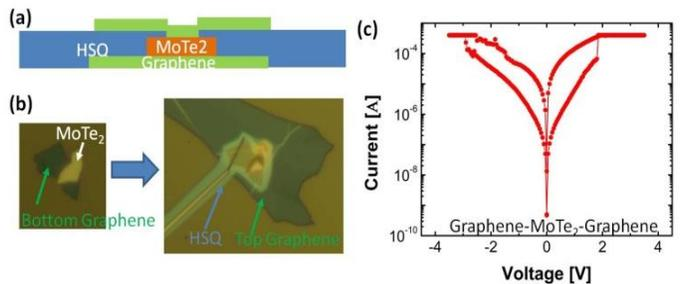
Fig. 7. (a) Schematic and (b) optical images of a Graphene-MoTe<sub>2</sub>-Graphene device. (c) I-V curve of the RRAM device in (b).
