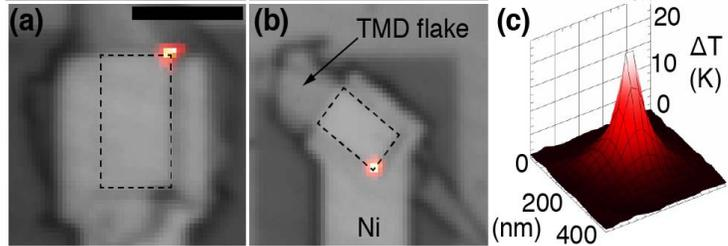
Fig. 4. (a-b) Thermoreflectance images showing the location of the filament. The scale bar is 5  $\mu$ m. (c) The calibrated temperature change map for the filament in the device (b).
