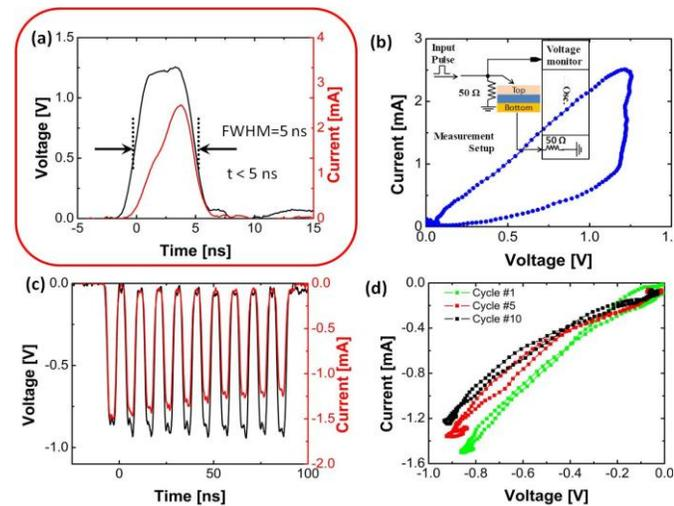
Fig. 10. (a) I/V vs. time plot showing switching of the device within a 5 ns voltage pulse. (b) I-V plot of the data shown in (a) to show the change in resistance during the applied pulse. The inset figure displays the experimental setup for the pulse measurement. (c) I/V vs. t plot of 10 reset pulses. (d) I-V plot of data plotted in (c) of pulses 1, 5 and 10.
