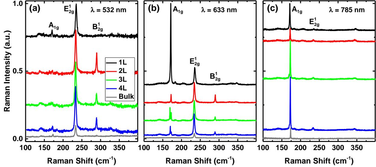
Figure S4: Raman spectra of 1L to 4L and bulk MoTe<sub>2</sub> (modes labeled according to bulk notation) using laser excitation wavelengths of (a) 532 nm, (b) 633 nm, and (c) 785 nm. The spectra are offset for clarity.
