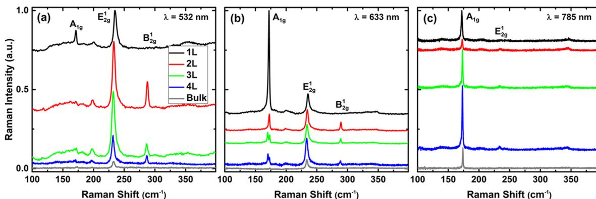
**Figure 2.** Raman spectra of 1L to 4L and bulk  $\text{Mo}_{0.91}\text{W}_{0.09}\text{Te}_2$  (modes labeled according to bulk notation) for excitation wavelengths of (a) 532, (b) 633, and (c) 785 nm. The spectra are vertically offset for clarity.
