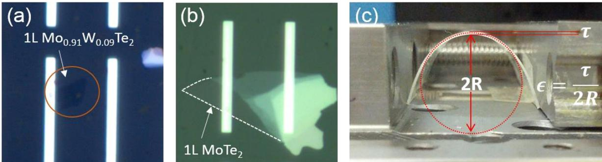
Figure S3: Optical image of (a) Mo<sub>0.91</sub>W<sub>0.09</sub>Te<sub>2</sub> and (b) MoTe<sub>2</sub> clamped to PEN with metal strips. (c) Two-point bending apparatus used for applying tensile strain. The strain is calculated from the formula shown, with the radius of curvature determined from the photo taken at each strain level.
