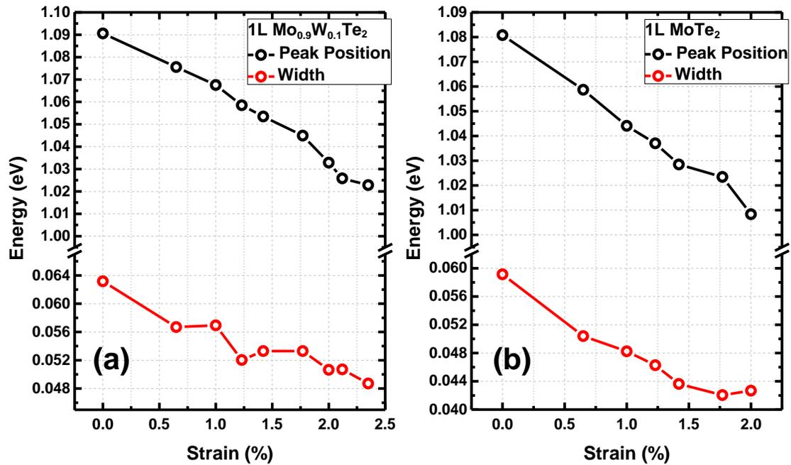
Figure S6: Peak positions and line widths of the strain-dependent PL spectra shown in Figure 4 in the main text for (a) 1L Mo<sub>0.91</sub>W<sub>0.09</sub>Te<sub>2</sub> and (b) 1L MoTe<sub>2</sub>.
