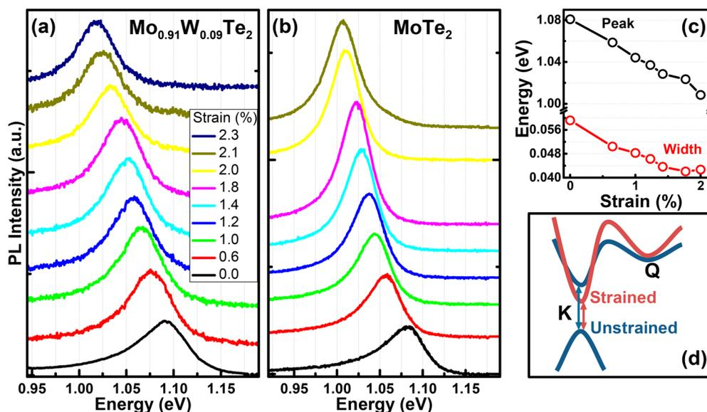
**Figure 4.** PL spectra of 1L (a)  $\text{Mo}_{0.91}\text{W}_{0.09}\text{Te}_2$  and (b)  $\text{MoTe}_2$  under different amounts of uniaxial tensile strain. All spectra are vertically offset for clarity. (c) Dependence of the peak energy and spectral width of 1L  $\text{MoTe}_2$  on strain. (d) Schematic band structure of strained and unstrained 1L  $\text{MoTe}_2$ , showing changes in the energy separation between the minima of the K and Q valleys in the conduction band.
