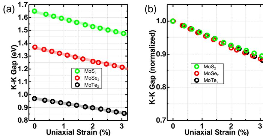
Figure S5: (a) Absolute and (b) normalized K-K gaps of  $\text{MoS}_2$ ,  $\text{MoSe}_2$ ,  $\text{MoTe}_2$  with increasing uniaxial tensile strain (adapted from the calculations by Rhim *et al.*<sup>10</sup>). The calculations suggest that band gaps of  $\text{MoS}_2$ ,  $\text{MoSe}_2$ , and  $\text{MoTe}_2$  redshift at a rate of about 55, 50, 37 meV/% strain, respectively.
