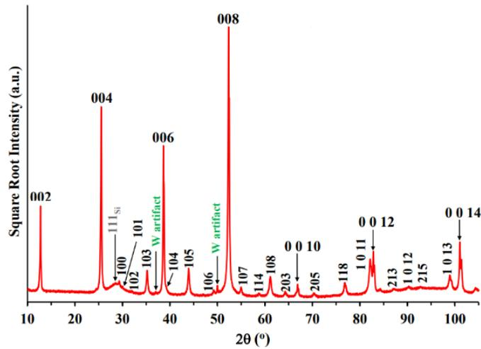
Figure S1: Extended version of the XRD scan for the  $\text{Mo}_{0.91}\text{W}_{0.09}\text{Te}_2$  sample, shown in Figure 1a in the main text. Experimental lattice parameters for the 2H crystal structure (space group  $P6_3/mmc$ ) are:  $a=3.5192(6)$  Å,  $c=13.9728(14)$  Å. These values agree with the literature data for  $\text{MoTe}_2$  compound:  $a=3.5182(14)$  Å and  $c=13.9736(40)$  Å.<sup>1</sup>
