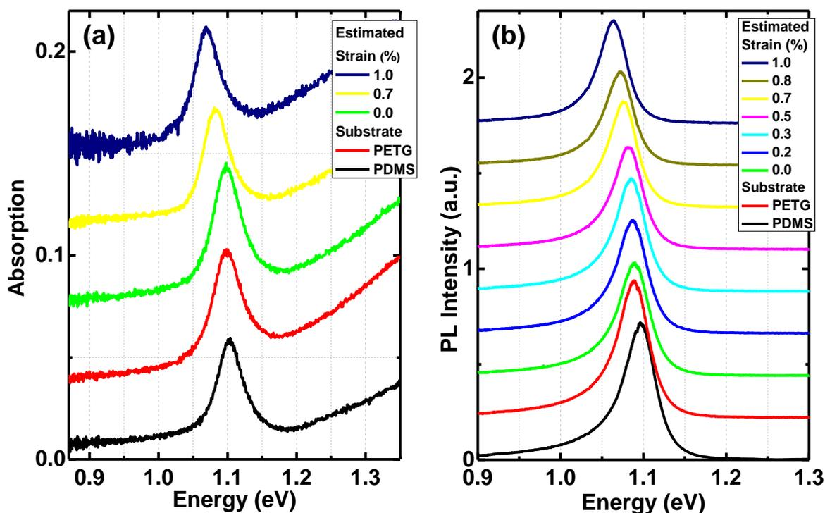
Figure S7: Strain-dependent (a) absorption and (b) PL measurements of 1L  $\text{Mo}_{0.91}\text{W}_{0.09}\text{Te}_2$  on PDMS (as-exfoliated, before transferring onto PETG), on PETG (after transfer) and with increasing strain. The spectra are vertically offset. Intensities of the measurements on PDMS were adjusted to match the PETG due to their different refractive indices which result in different electric field enhancement on their surfaces.
