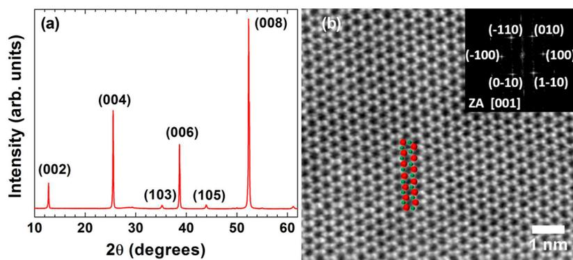
**Figure 1.** (a) Powder XRD pattern of  $2\text{H-Mo}_{0.91}\text{W}_{0.09}\text{Te}_2$ . (b) High angle annular dark field scanning electron microscopy (HAADF-STEM) image of a  $2\text{H-Mo}_{0.91}\text{W}_{0.09}\text{Te}_2$  sample together with an overlapped structural model: red (large) spheres, Mo/W atoms; green (small) spheres, Te atoms. Inset: fast Fourier transform (FFT) emphasizing the  $[001]$  zone axis.
