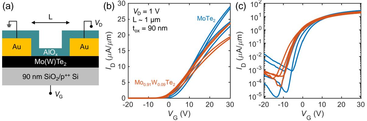
Figure S9: (a) Device cross-section diagram. (b) Linear and (c) log scale plots showing measured drain current ( $I_D$ ) vs. gate voltage ( $V_G$ ) transfer curves of two few-layer  $\text{Mo}_{0.91}\text{W}_{0.09}\text{Te}_2$  (red) and two few-layer  $\text{MoTe}_2$  (blue) transistors with channel lengths of  $\sim 1 \mu\text{m}$ . The double curves show the forward and backward  $I_D$ - $V_G$  sweeps.
