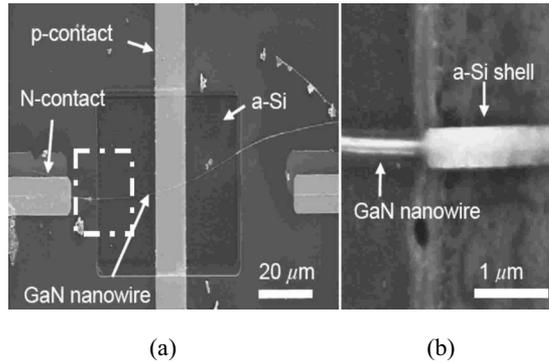
FIG. 2. (a) SEM image of a completed GaN/a-Si heterojunction diode. (b) High-magnification SEM image of the area highlighted in (a) by broken white square showing the core-shell nature of the completed device.
