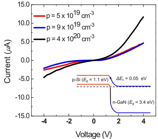
FIG. 3. (Color online) Room-temperature *I*-*V* characteristics of three different GaN nanowire/Si core-shell diodes with three doping levels of the *p*-Si shell. Diameters of the nanowires were in the range of 180–200 nm. (Inset) Equilibrium band alignment of *p*-Si and *n*-GaN.
