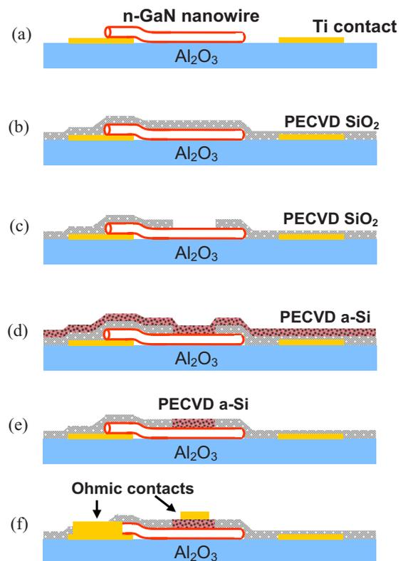
FIG. 1. (Color online) Schematic representation of the fabrication process of GaN/*a*-Si core-shell structure.
