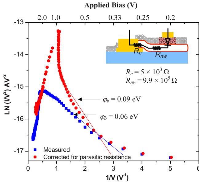
FIG. 5. (Color online) Plot of  $\ln(I/V^2)$  vs  $1/V$  (forward bias regime) showing the straight-line fit of the data at low voltage regime. The blue curve is for the measured data and red is for the data corrected for the parasitic series resistances. (Inset) The lumped model showing the parasitic resistances and their estimated values.
