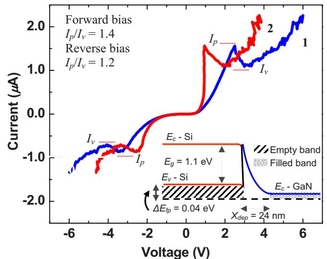
FIG. 4. (Color online) Room-temperature *I*-*V* characteristics of a single GaN nanowire/*a*-Si junction exhibiting NDR. The blue curve (1) is measured data and the red curve (2) is corrected for parasitic series resistance. (Inset) Equilibrium band alignment of *p*-Si and *n*-GaN showing only the alignment of Si band edges with conduction band of GaN, where  $\Delta E_{fp}$  is the relative Fermi level for Si given by  $(k_B T/q) \ln(N_v/p)$ .
