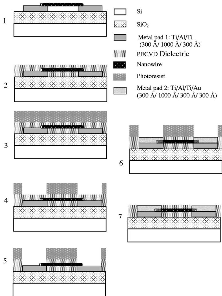
FIG. 3. Schematic representation of the fabrication process flow.
