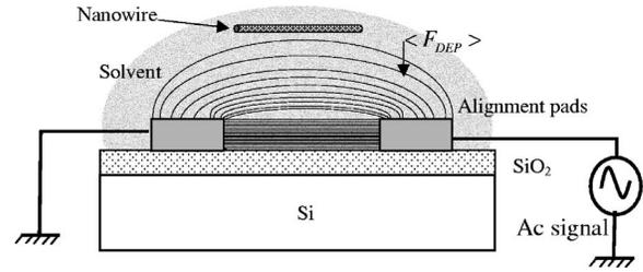
FIG. 1. Schematic representation of the dielectrophoretic alignment of nanowires using a solvent medium.
