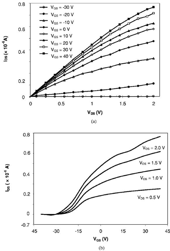
FIG. 13. (Color online) (a) Plot of  $I_{DS}$  vs  $V_{DS}$  of a nanowire device of type II (diameter of 95 nm and length of 35  $\mu\text{m}$ ) with  $V_{GS}$  varied from  $-30$  to  $+40$  V. (b) Transconductance plot of the same nanowire device ( $I_{DS}$  vs  $V_{GS}$ ) for different  $V_{DS}$ . The device could be completely turned off at  $-30$  V  $V_{GS}$ .
