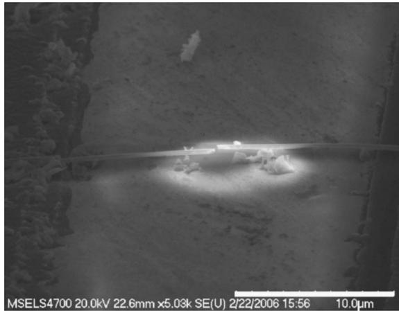
FIG. 11. FESEM scan of the nanowire device ( $I$ - $V$  characteristics present in Fig. 10) after annealing of the second metal stack. The break in the nanowire is clearly visible, which might be caused by the thermal stress during annealing. This nanowire is assembled on a sapphire substrate with no PECVD protective oxide coating.
