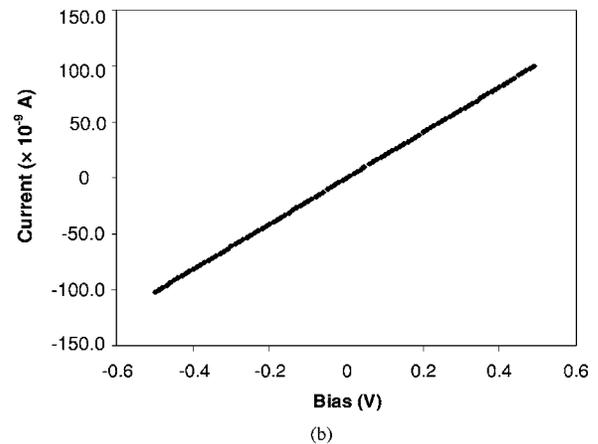
FIG. 10. (a)  $I$ - $V$  characteristics of a single nanowire (110 nm diameter and  $30\ \mu\text{m}$  in length) with the as-deposited second metal stack. (b)  $I$ - $V$  characteristics of the same nanowire after annealing the second metal stack showing significant deterioration.
