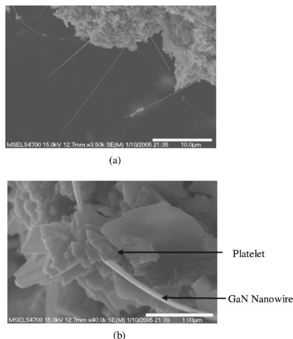
FIG. 4. (a) FESEM scans of the growth matrix after collecting from the growth chamber. (b) FESEM scans of nanowires growing from the edges of the GaN platelets.
