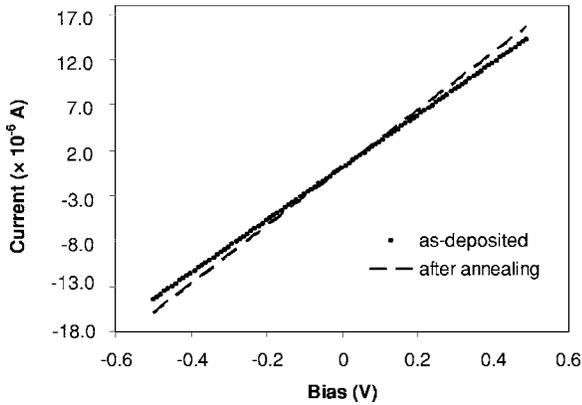
FIG. 8.  $I$ - $V$  characteristics of a single nanowire (100 nm diameter and  $35\ \mu\text{m}$  in length) with the as-deposited second metal stack (—) and after annealing (---).
