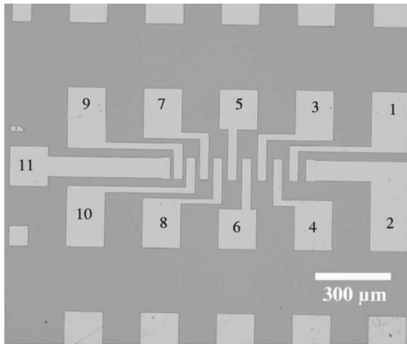
FIG. 2. Typical Ti/Al/Ti alignment pads on SiO<sub>2</sub>/Si substrate. The spacings between the interdigitated electrodes varied from 14  $\mu\text{m}$  at the one end (between electrodes 11 and 9) to 28  $\mu\text{m}$  at the other end (between electrodes 2 and 1).
