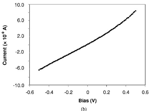
FIG. 9. (a)  $I$ - $V$  characteristics of a nanowire with the as-deposited second metal stack showing nonlinear behavior with the lower current levels. (b)  $I$ - $V$  characteristics of the same nanowire after annealing the second metal stack.
