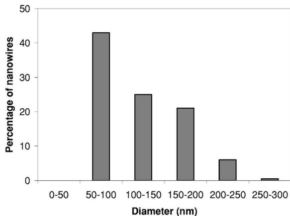
FIG. 5. Diameter distribution of nanowires as observed in the growth matrix.
