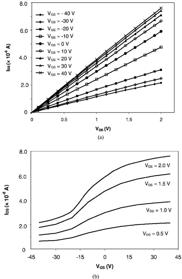
FIG. 12. (a)  $I_{DS}$  vs  $V_{DS}$  plot for a nanowire device of type I (diameter of 200 nm and length of  $44 \mu\text{m}$ ) with  $V_{GS}$  varied from  $-40$  to  $+40$  V. (b) Transconductance plot of the same nanowire device ( $I_{DS}$  vs  $V_{GS}$ ) for different  $V_{DS}$ .
