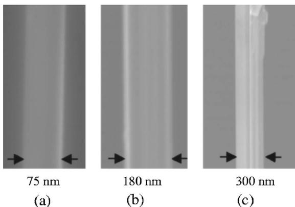
FIG. 6. Representative structural characteristics of nanowires observed in different diameter ranges: (a) 50–100 nm, (b) 150–200 nm, and (c) 250–300 nm. Diameters of the nanowires are indicated below.
