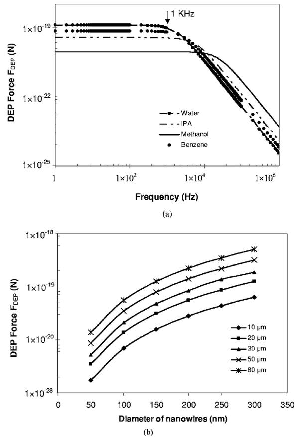
FIG. 14. (a) Calculated DEP force experience by a nanowire (100 nm diameter and 50  $\mu\text{m}$  in length) in different dispersing media as a function of the alignment voltage. The drop in the DEP force for different solvents starts around 1 kHz. (b) Calculated DEP force variation as a function of nanowire diameter and length. The alignment frequency is set to 1 kHz and the dispersing medium is IPA.
