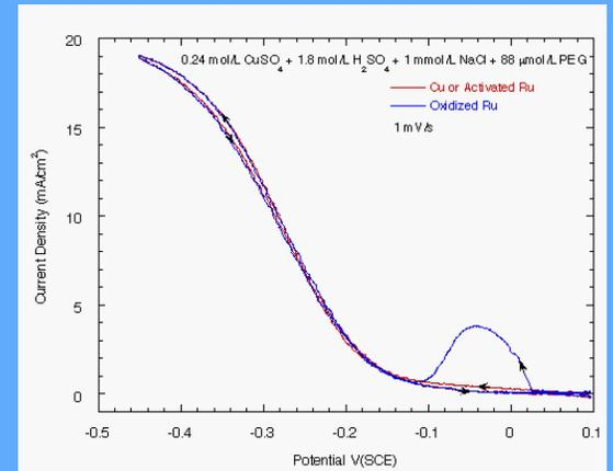
Process based on hydrogen reduction of surface oxide. (Moffat, ECS, Spring 2005).
