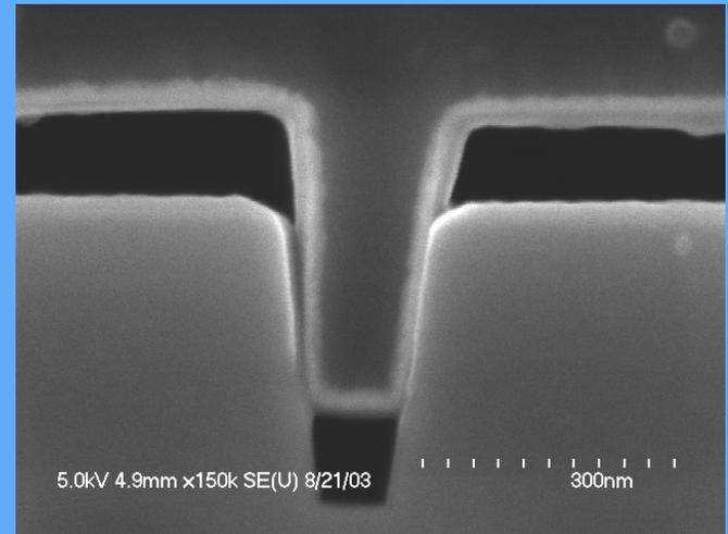
Adhesion of ALD Ru barrier to the TEOS dielectric was poor with an intervening water pulse (meant to create hydroxyl bonds) rather than the alumina adhesion layer.
