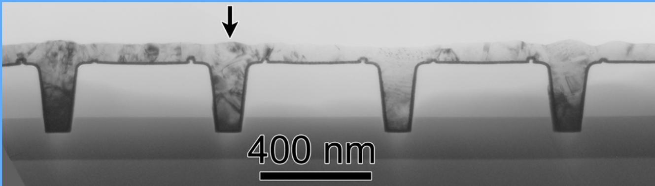
Recrystallization of the Cu conductor is qualitatively similar to that observed on Cu seeded barriers.
