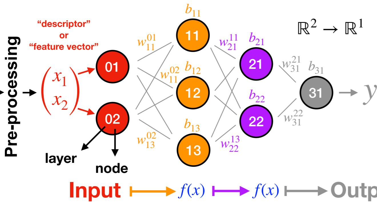
**Hidden layer-1 output**  $\mapsto \begin{pmatrix} O_{11} \\ O_{12} \\ O_{13} \end{pmatrix} = f \left( \begin{pmatrix} w_{11}^{01} & w_{11}^{02} \\ w_{12}^{01} & w_{12}^{02} \\ w_{13}^{01} & w_{13}^{02} \end{pmatrix} \begin{pmatrix} x_1 \\ x_2 \end{pmatrix} + \begin{pmatrix} b_{11} \\ b_{12} \\ b_{13} \end{pmatrix} \right) \rightarrow$  **apply activation function component wise**
