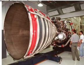
The upgraded Block 2 engine sits in the Space Shuttle Main Engine Processing Facility at Kennedy Space Center awaiting transfer to Atlantis' hangar
