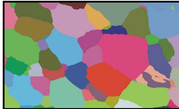
dolomite marble microstructure
