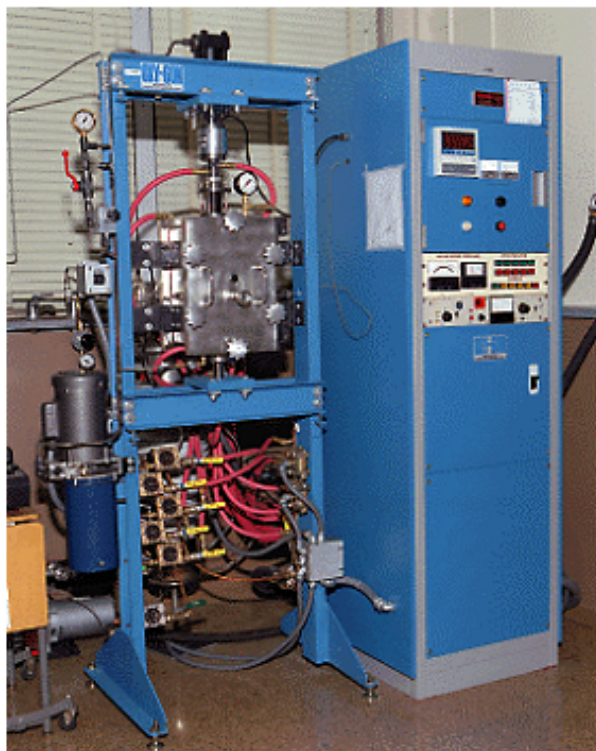
The vacuum/inert gas hot press unit to be used to fabricate the superalloys / Ni couples
