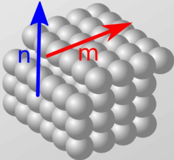
Accumulated slip of the plane with normal **n** in the direction **m** contributes to the plastic strain rate by the outer product of **m** and **n**.
