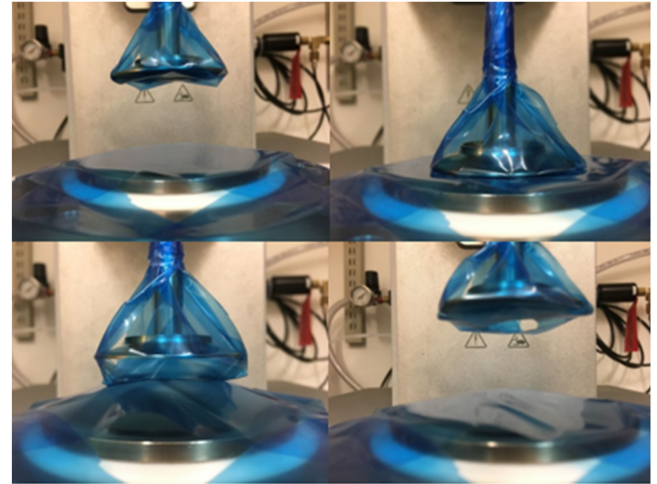
Fig. 2. The rheometer with wafer dicing tape attached as it exfoliates \text{MoTe}_2 crystals. (Top left) The rheometer plate descending towards the stage; (top right) the plate as it contacts the stage; (bottom left) the plate as it ascends from the stage; (bottom right) the plate after completing one cycle of exfoliation.
