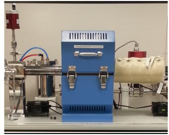
**Figure S2.** Photograph of the PlanarTECH custom 2-inch tube furnace used to grow MoSe<sub>2</sub>, corresponding to the diagram in Figure S1.
