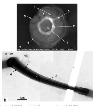
Fig. 3 (a) FESEM, a NW-LiB's cross-section. (b) BF-TEM montage, a NW-LiB contacted with Pt pads, a cut was made by DB-FIB to reduce the leakage through the supporting silicon nitride membrane. (1) (111) Si NW, (2) Ti/Pt/Ti metal collector layer, (3) platelet-like LiCoO<sub>2</sub> crystallites in the cathode layer, (4) LiPON electrolyte layer, (5) n-Si amorphous anode layer, (6) voids.
