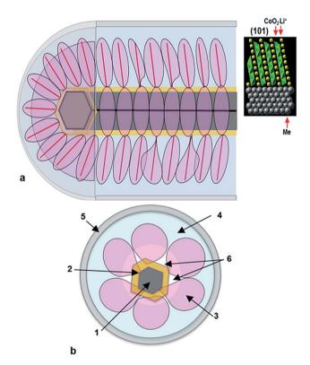
Fig. 7 Schematic of a NW-LIB showing its 3D morphological and structural arrangement: (a) *Y*-section, an enlarged view of the LiCoO<sub>2</sub>-metal collector interface (inset). (b) *X*-section. Red lines parallel to (003) planes indicate directions of preferential growth of LiCoO<sub>2</sub> platelet-like nanocrystallites. (1) (111) Si NW, (2) metal collector layer, (3) LiCoO<sub>2</sub> cathode layer, (4) LiPON electrolyte layer, (5) *n*-Si amorphous anode layer, (6) voids.
