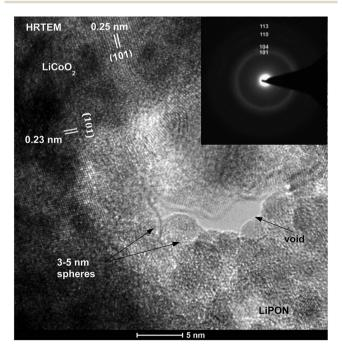
**Fig. 9** HRTEM of a thin NW-LiB thin section. The area around the void reveals 5 nm to 10 nm  $\text{Li}_{1-x}\text{CoO}_2$  crystallites with 0.25 nm (101) lattice fringes and 3 nm to 5 nm diameter amorphous particles. SAED pattern (right inset) displays broadened (101), (104), (110) and (113) ring reflections.
