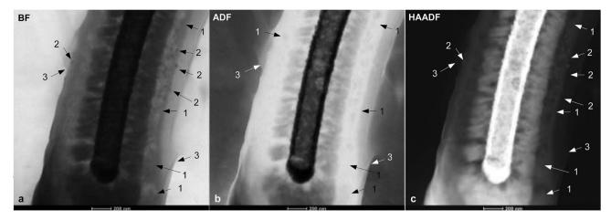
**Fig. 8** *Ex situ* STEM, a cycled NW-LiB after 8<sup>th</sup> discharge. (a) BF-STEM. (b) ADF-STEM. (c) HAADF-STEM. 50 to 100 nm voids (1) at and near the LiPON-Li<sub>1-x</sub>CoO<sub>2</sub> interface, 10 to 40 nm spherical particles (2) located in the LiPON layer and partially delaminated 10 to 50 nm thick *n*-Si anode layer (3) are evident.
