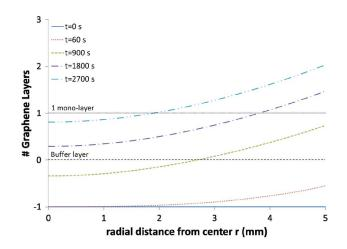
Fig. 9. Plot of the time-dependent solutions for the graphene layer coverage, with a bare SiC surface being -1, at five points in time and an annealing temperature T = 1900 °C, as described in the text.
