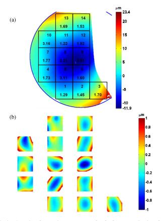
Fig. 3. Laser interferometric measurement of wafer flatness: (a) Section of Si face of a 50-mm SiC wafer, with the measured flatness deviation in false color. Each 8 mm  $\times$  8 mm sample area is identified by a sequential number and its peak-to-valley flatness error; (b) flatness deviation of each sample area.
