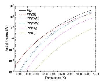
Fig. 1. Equilibrium partial pressure above a bare 6H-SiC surface, calculated using ThermoCalc<sup>®</sup>.<sup>1</sup> Note that Si and Si<sub>2</sub>C are the dominant vapor species, which results in the incongruent sublimation of silicon carbide and formation of graphene layers.
