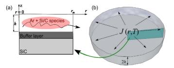
Fig. 7. Geometry of the problem. J(r, T) is the gas flux, r the radial distance,  $r_m$  is the maximum radius, T is the temperature, and 2h is the gap height. (a) Cross section as indicated, after the BF growth, (b) we assume a cylindrical geometry for the gas to diffuse. Image dimensions are not to scale ( $r_m \approx 4 \text{ mm}$ ;  $h \approx 1 \mu \text{m}$ ).
