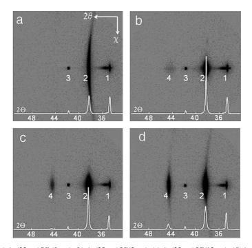
Fig. 2. XRD patterns for: (a) Au(35 nm)/Ni (0 nm); (b) Au(35 nm)/Ni(5 nm); (c) Au(35 nm)/Ni(15 nm); (d) Au(35 nm)/Ni(65 nm). Angular integrated "intensity  $-2\theta$ " scans (solid white lines) are superimposed on two-dimensional  $2\theta - \chi$  GADDS images. Reflections: (1) GaN 0002; (2) Au 1 1 1; (3) Al<sub>2</sub>O<sub>3</sub> 0 0 0 6; (4) Ni 1 1 1.
