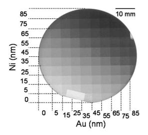
Fig. 1. Au/Ni metallization library deposited on GaN/sapphire. Numbers indicate nominal Ni and Au thicknesses for each metallization element in the array.
