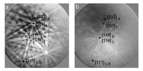
Fig. 4. EBSD patterns from: (a) Au(35 nm)/Ni(5 nm); (b) Au(35 nm)/Ni(65 nm). Indices with subscripts I and II indicate presence of two Au domains, related by 60° rotation about [1 1 1]. Note loss of contrast in pattern (b) due to increased grain misorientation in Au/Ni layers.
